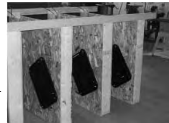
A stationary RFID reader designed for the Wisconsin RFID project. This was one of five reading systems used in the project, including stationary readers and handheld wands. The study found that the technology may not be ready for use by most producers.
